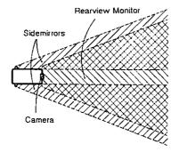
Note that the left and right sides of the image on the monitor are reversed, just like that of the rearview mirror.
