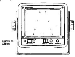
Whenever changing the gear shift lever to the reverse position, the Mode Indicator LED turns to amber (ON mode) and the rearview picture can automatically be seen on the monitor screen in a few seconds.
