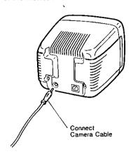
Connect the supplied remote cable to the power source and to the remote connector (DC IN/REMOTE) on the rear of the monitor.
