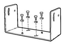
Secure the monitor onto the monitor fixing bracket by using the supplied 4 monitor fixing screws and adjust the tilt of the monitor.
