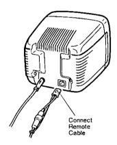
Connect the +12V/24V wire (Red) to the +12V/24V line which is electrically after the ignition switch, the remote input wire (Blue) to the +12V/24V line for the reverse light and the ground wire (Green) with lug to the chassis of the vehicle.
